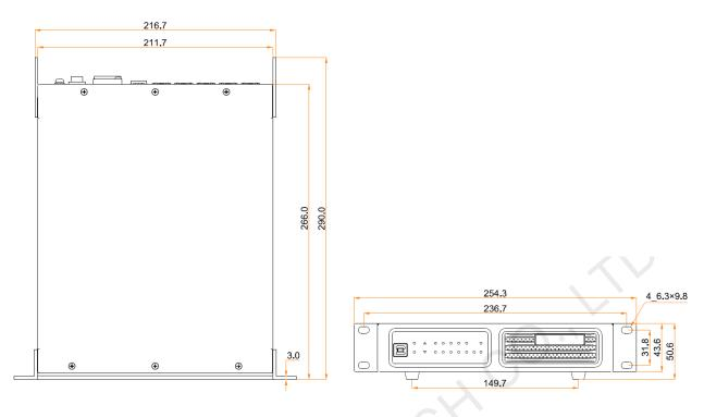
Tolerance: ±0.3 Unit: mm
