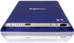
Offers our most powerful H.264/H.265 4K & Full HD video engine with Dolby Vision and HDR10 support, 4K full resolution graphics, 4K upscaling and dual decoding of two 4Kp60 videos simultaneously. Delivers the best HTML5 rendering performance available for Enterprise applications. Includes the standard I/O package of Gigabit Ethernet with PoE+, GPIO, IR, analog/digital audio and an M.2 SSD PCIe interface.
