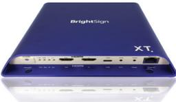
Includes all the features BrightSign XT244, plus serial, dual USB (type A and C) and Live TV playback via the HDMI 2.0a input to play content from any broadcast channel – even protected HDCP content.
